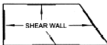
Fig.2.5.4e Non-parallel Systems of Shear Wall
